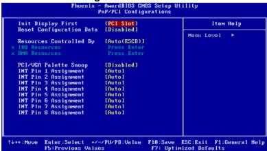
**NOTE:** This "PnP/PCI Configurations" option is setting up the IRQ and DMA (both PnP and PCI bus assignments.
